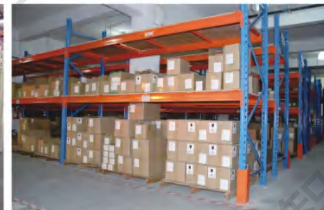
貨架鋪木板案例 Case of rack with plywood
