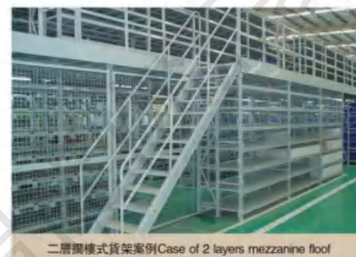
二層擱樓式貨架案例 Case of 2 layers mezzanine floor
