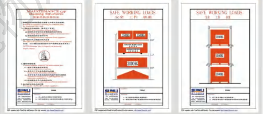
安全標識 Signs containing basic safety rules and recom--mended loading limits should be prominently displayed within the operating area of the racking.
