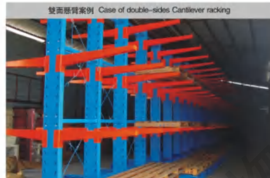
雙面懸臂架 Case of double-sides Cantilever racking
