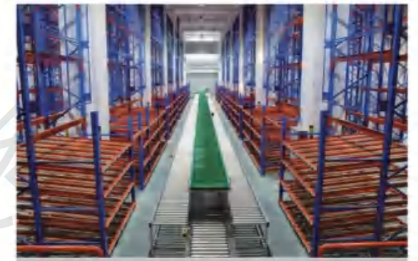
流利架細節展示 The detail showing of gravity racking
