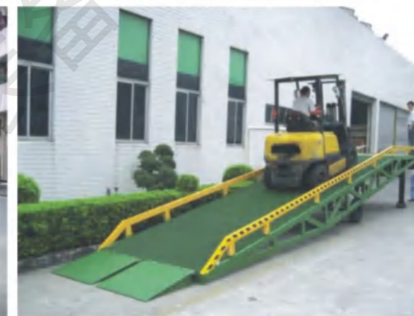
承載測試中移動登車橋 Loading capacity test-mobile ramp
