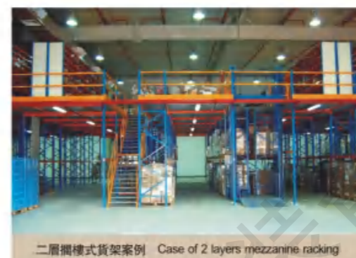
二層擱樓式貨架案例 Case of 2 layers mezzanine racking
